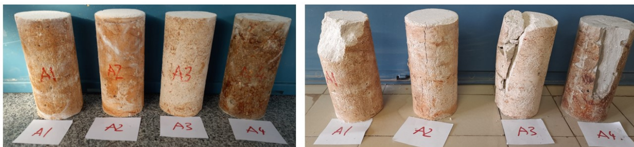
Figure 7: Before test and after test images of plaster samples
