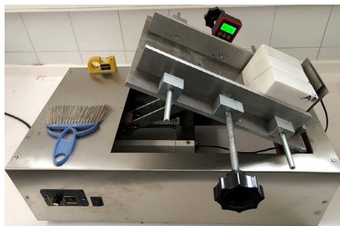
Figure 2. Tilt device used in experimental studies
