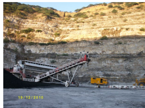
Figure 8. View of ADDCAR-make Highwall Mining machine in operation at SCCL
