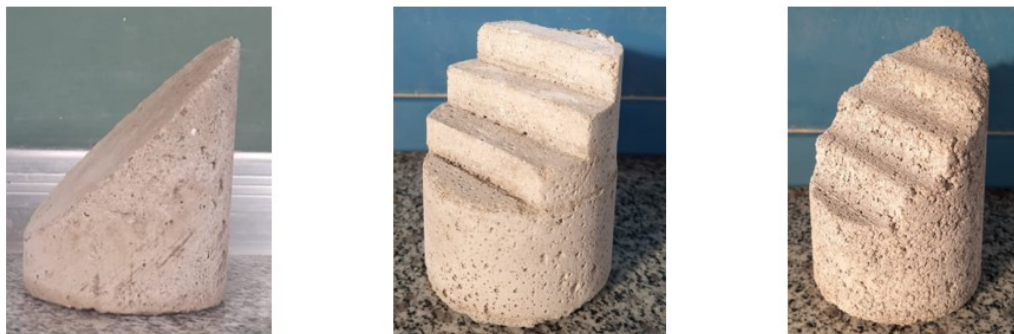
Figure 4: The concrete samples prepared with the help of 3D printed molds
