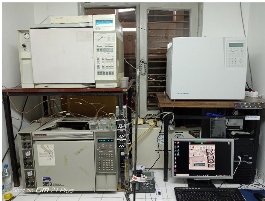
Figure 8. A photograph from the laboratory built for the determination of formaldehyde content of phenol-based filling materials (See Headspace Perichrom GC, right up) (See GC-FID left up).
