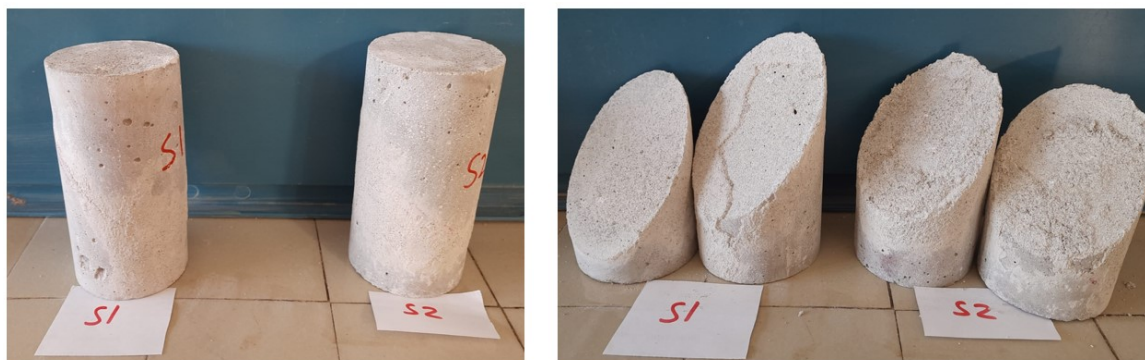
Figure 8: Before test and after test images of concrete samples with smooth discontinuity planes
