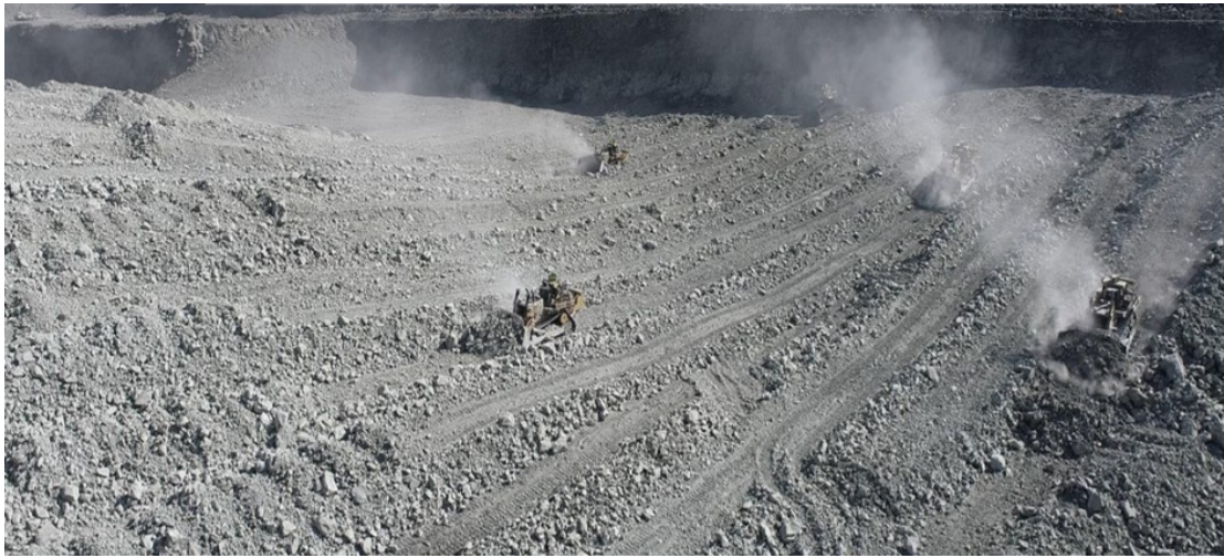
Figure 1. Typical Bulk Dozing in an Opencut mine
