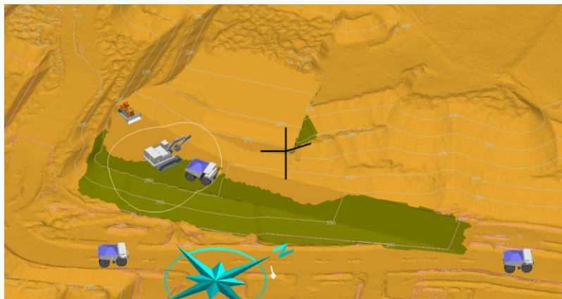
Figure 14. Modelling Dozing in 3DDig (Post-Doze surface)
