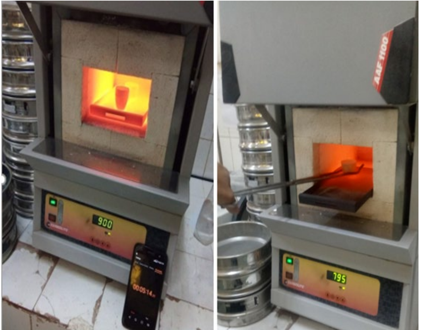
Figure 4. Muffle furnace used in the test
