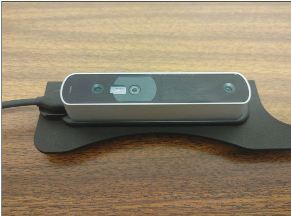
Figure 2. Occipital Structure Sensor (Mark II)
