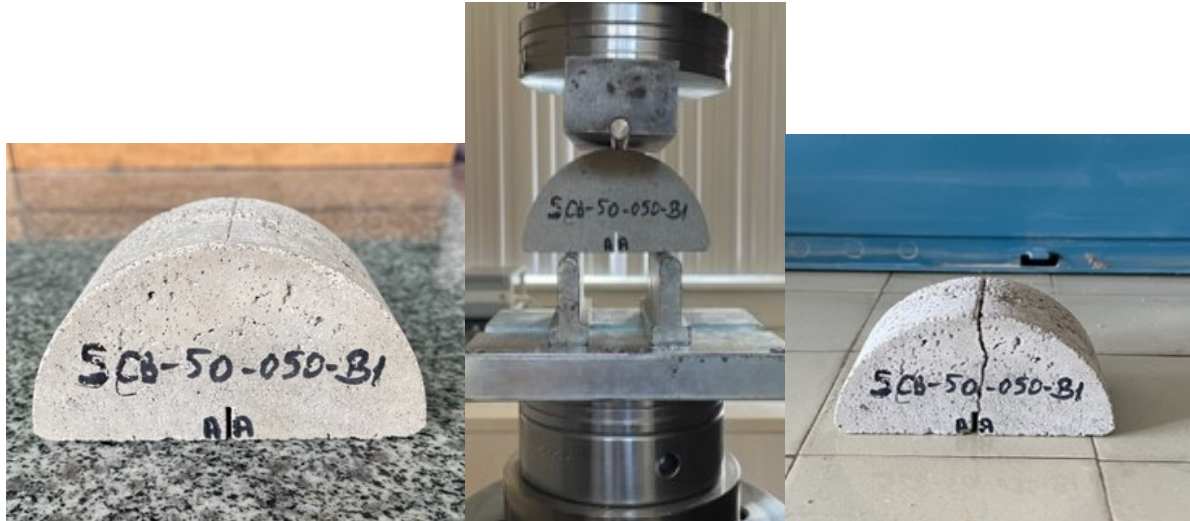
Figure 5. SCB sample before, during and after the test
