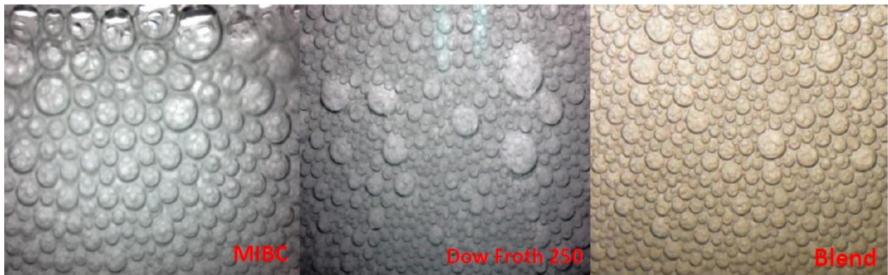
Figure 2. The images of MIBC, Dowfroth 250 and their blend at 50 ppm concentration
