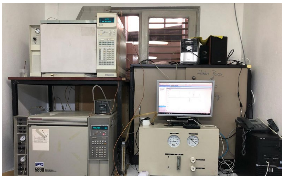
Figure 6. Spontaneous combustion experiment set up, HP 5890 (employed only as an oven, left bottom) and HP 6890 (employed as GC-FID, left up) (Adapted from the study of Bilen et al. 2019).
